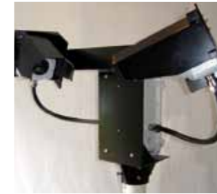
Scattering angle 42 degree scattering angle ensures accurate measurement
