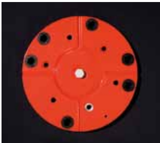
Installation The bottom plate of the LDR 155 EX supports installation on structure using 3 x M12 bolts or 4 x M12 bolts on a 200 mm radius. The mounting holes are galvanic isolated with plastic isolators. PTFE breathing vent for pressure release.
