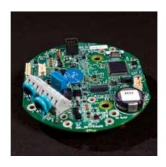
Sabik Marine Controller (SMC) is the lantern integrated controller (flasher). The SMC comes with all the proven solutions invented by Sabik for the previous generation controllers. A wide range of innovative functions are included and we are setting a new standard for efficiency of flashers.
